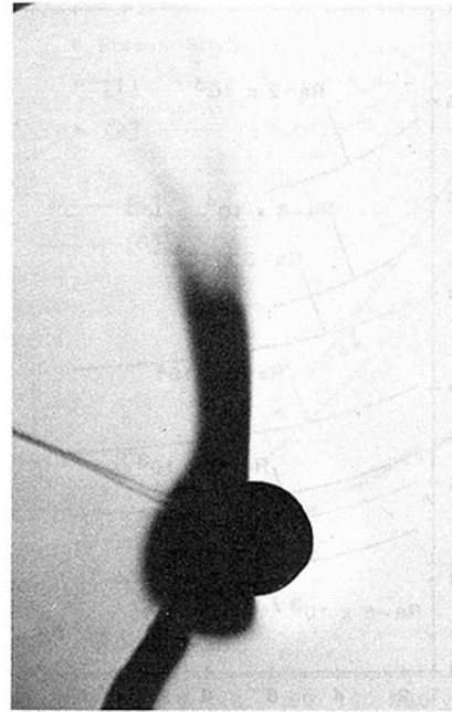
Fig. 8(a) Schlieren photograph for the unconfined heated cylinder, Ra = 5 \times 10^4 , W/D = \infty
